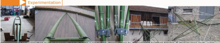
Compression bars were then built at a scale of 1/1, during a workshop stage, where bi-dimensional bamboo beams, 5 meters long each, were profiled. This step allowed us to test structural behaviour (with resin reinforcing at the end of bars, and metallic assemblies for cable links). A tensegrity tripod could then be erected, (with nylon tape for industrial packaging as tension elements), its resistance was tested for a few days
